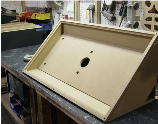
Fig 5: Intermediate plate in enclosure
